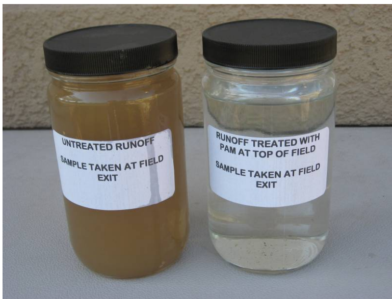
Figure 22. Comparison of runoff samples taken at field exit with and without the use of PAM.
