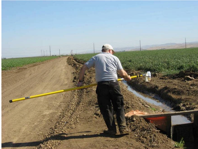
Figure 10. Sampling of Weir Located at Edge of Field and prior to the Sediment Basin
